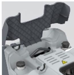
access to crossbar and tanks filling
