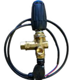
VRT3 Panel Mount Unloader + Press SW 250 bar 3/8" F inlet 40 L/min 3/8" F outlet 2 x 1/4" BSPF bypass Part No: PWP6/5
