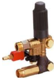
Unloader Control Set Chemical injector & bypass 200 bar 11-15 L/min 1/2" F inlet 3/8" M outlet Part No: W2L-1
