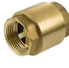
Non-Return Valve 2"F - 2"F Max. 25 bar Max. 50°C
