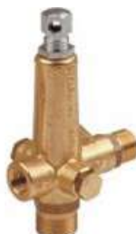
K3.1 Unloader Valve 100 bar 3/8" F inlet 11-16 L/min 1/2" M outlet 1/2" F & 3/4" M bypass
