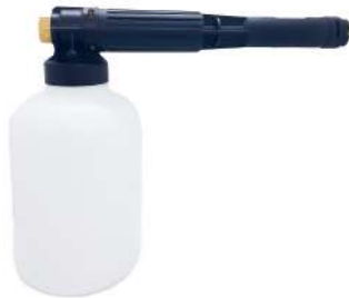
PA Foam Injector Head inc. 2L bottle 200 bar 1/4" M inlet 20 lpm 60°C max. Part No: PWP58/13
