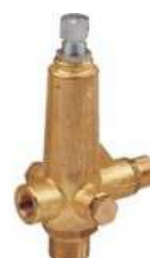
K5 Unloader Valve 200 bar 3/8" F inlet 11-16 L/min 1/2" M outlet 1/2" F & 3/4" M bypass
