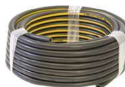
Low Pressure Hose 3/4" order per metre Max. 20 bar / 90°C Part No: PWPH132
