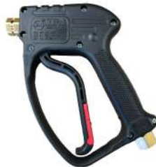
RL30 + Swivel 345 bar 3/8" F inlet 40 L/min 1/4" F outlet 160°C inc. swivel
