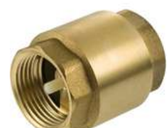
Non-Return Valve 1 1/2"F - 1 1/2"F Max. 25 bar Max. 50°C
