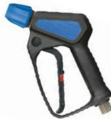
ST2300S Trigger Gun 310 bar 3/8" F inlet 45 L/min QR F outlet 150°C
