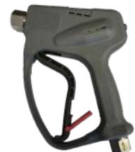
RL84 Trigger Gun 500 bar 1/2" F inlet 80 L/min 1/2" F outlet 100°C Stainless Steel
