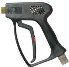
ST1500 + Swivel 275 bar 3/8" F inlet 45 L/min 1/4" F outlet 160°C inc. stainless steel swivel
