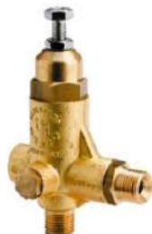
K1 Unloader Valve 250 bar 3/8" F inlet 9-41 L/min 1/2" M outlet 1/2" BSPM bypass
